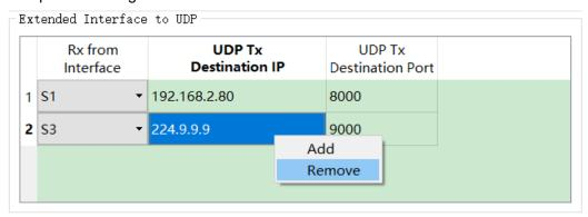
According to the application requirements, 'UDP send destination IP address' can be unicast, multicast or broadcast address.
