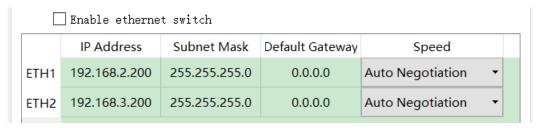
With the dual-IP function figure as follows, the MVB-TCMS is equivalent to a PC equipped with two network cards.
