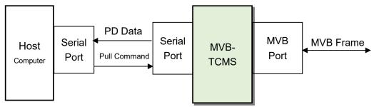
When the serial port works in the RS-232/422 full-duplex mode, the sending and receiving operations of the serial port can be carried out at the same time without conflict. The MVB can be transferred to the serial port by periodic active sending or pulling mode.
