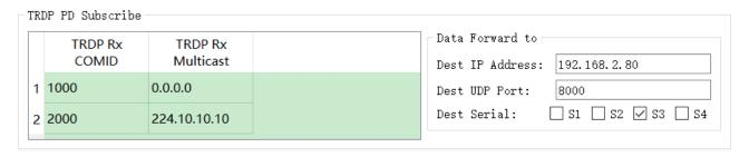
As shown above, the subscription TRDP PD data is forwarded to the serial port S3 and the host with the destination IP of 192.168.2.80, where COMID 2000 is received through multicast.
