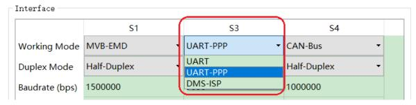
After determining the working mode, the contents of the "Advanced Options" cell will be adjusted automatically according to the working mode.
