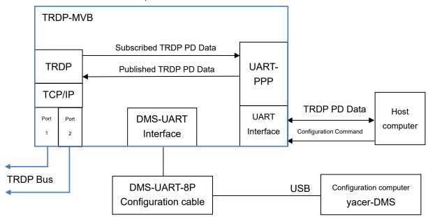
For reliable data transmission with the host computer through the UART interface, the TRDP-MVB uses the UART-PPP protocol to encapsulate the data.
