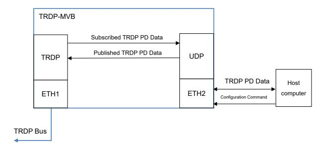
At the same time, the host computer can run the yacer-DMS configuration management software to manage the configuration of TRDP-MVB via Ethernet.
